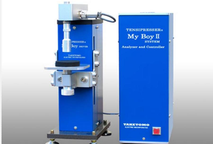
Fig.12 物性測定機TENSIPRESSER (TTP-50BX II 2006: TAKETOMO)
